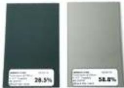
When testing with the calibration standards, conduct your measurement in the same manner as testing an actual window. When not in use, store the calibration standards in the re-sealable bag they were packaged in, and keep them inside the carrying case for best protection. If the calibration standards become scratched or damaged, replacement sets can be ordered from the manufacturer. The part number for the replacement standard set is TC3811.
