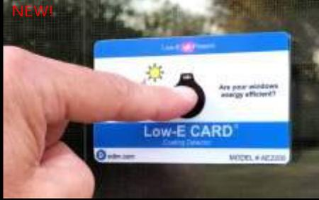
Low-E CARD® COATING DETECTOR - DISPOSABLE (#AE2200)
