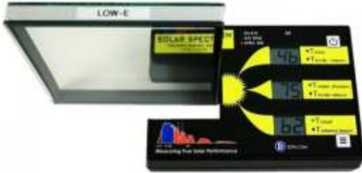
Solar Spectrum Transmission Meter Full spectrum measurements Values calculated to 3 standards Tuv, Tvis, Tsolar, Tir & Tdw
