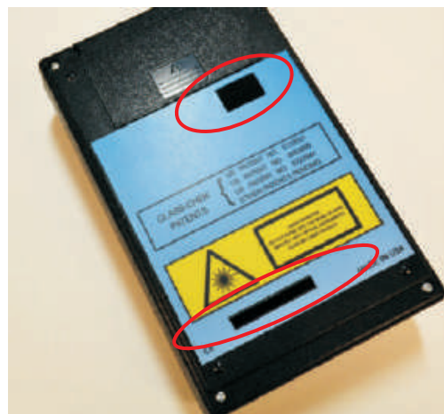
Above: Back of GC3200 meter with the two lenses circled. Use clean compressed air to clean the lenses.
