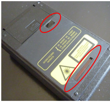
Figure 2: Back of GC3000 meter with the two lenses circled. Use clean compressed air to clean the lenses.
