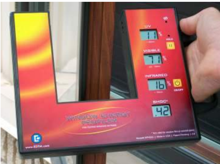
At left: Testing with the WP4500 Window Energy Profiler.
